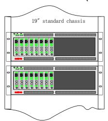
Note: Brackets used to fix the chassis are in the accessory box. If you use the bracket's rear holes to attach brackets to the chassis, there will be 3cm space between chassis front panel and cabinet front panel; and if you use the bracket's front holes, the front panel and the rack will be at the same level vertically.
